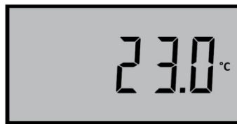
Waiting to START Press START button continuously for 5 seconds to start the logger.
