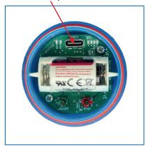
Any USB Type-A to USB Type-C data cable can be used to connect the logger to its USB Type-C port.
