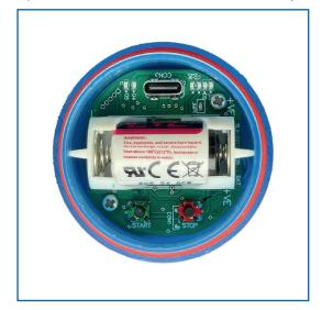
Press and hold the STOP button for 5 seconds until the red «D3» LED turns on.
