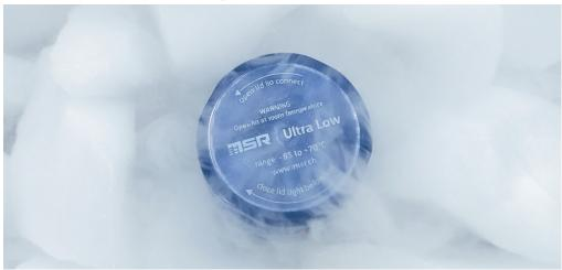
The robust MSR85 data logger ensures reliable temperature monitoring for products transported or stored with dry ice. It is ideal for sensitive goods such as pharmaceuticals, vaccines, biological samples, tissues or enzymes that require a secure cold chain down to -85 °C.
